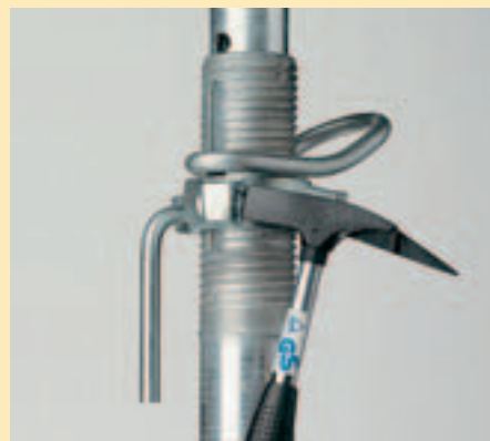
Lowering with the directional adjusting nut, easy on the materials.
